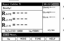
Press **F1**  $U_N$  push-button and move to selection of test voltage  $U_N$ .
