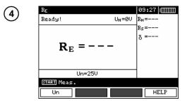
The meter is ready for measurement. Value of interference voltage  $U_{\rm N}\,{\rm can}$  be read on the display.
