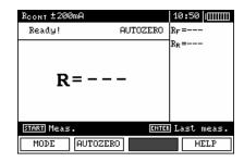
**AUTOZERO** message appears that confirms completion of test leads calibration.
