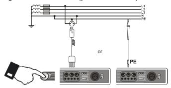
When the meter is connected according to the drawing, touch the touch electrode with a finger and wait for about 1 second. When voltage if found on PE, the device displays **PE!** message (error in the installation; PE lead is connected to the phase lead) and generates a continuous audio signal. This possibility is available for all measuring functions that apply to residual current devices (RCD) and short circuit loop.
