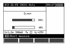
Progress of measurement process is shown by progress bars: lower bar – total cycle; upper bar – measurement of  $Z_{L\text{-PE}}$  RCD and  $I_A$ .
