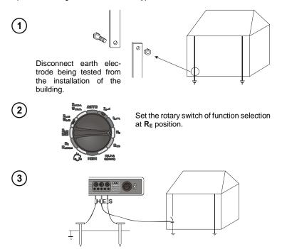
The current electrode (driven into earth) should be connected to **H** socket of the meter. The voltage electrode (driven into earth) should be connected to **S** socket of the meter. The earth electrode being tested should be connected to **E** socket of the meter. The earth electrode being tested and the current electrode and the voltage electrode should be
