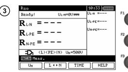
Press F1  $U_N$  push-button and move to selection of test voltage  $U_N$ .
