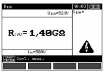
View of the screen during measurement performed with the use of **ENTER** pushbutton.
