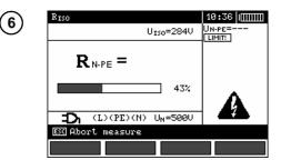
View of the screen during measurement. Symbol of the resistance being measured is displayed. Progress bar shows % of progress of total measurement.
